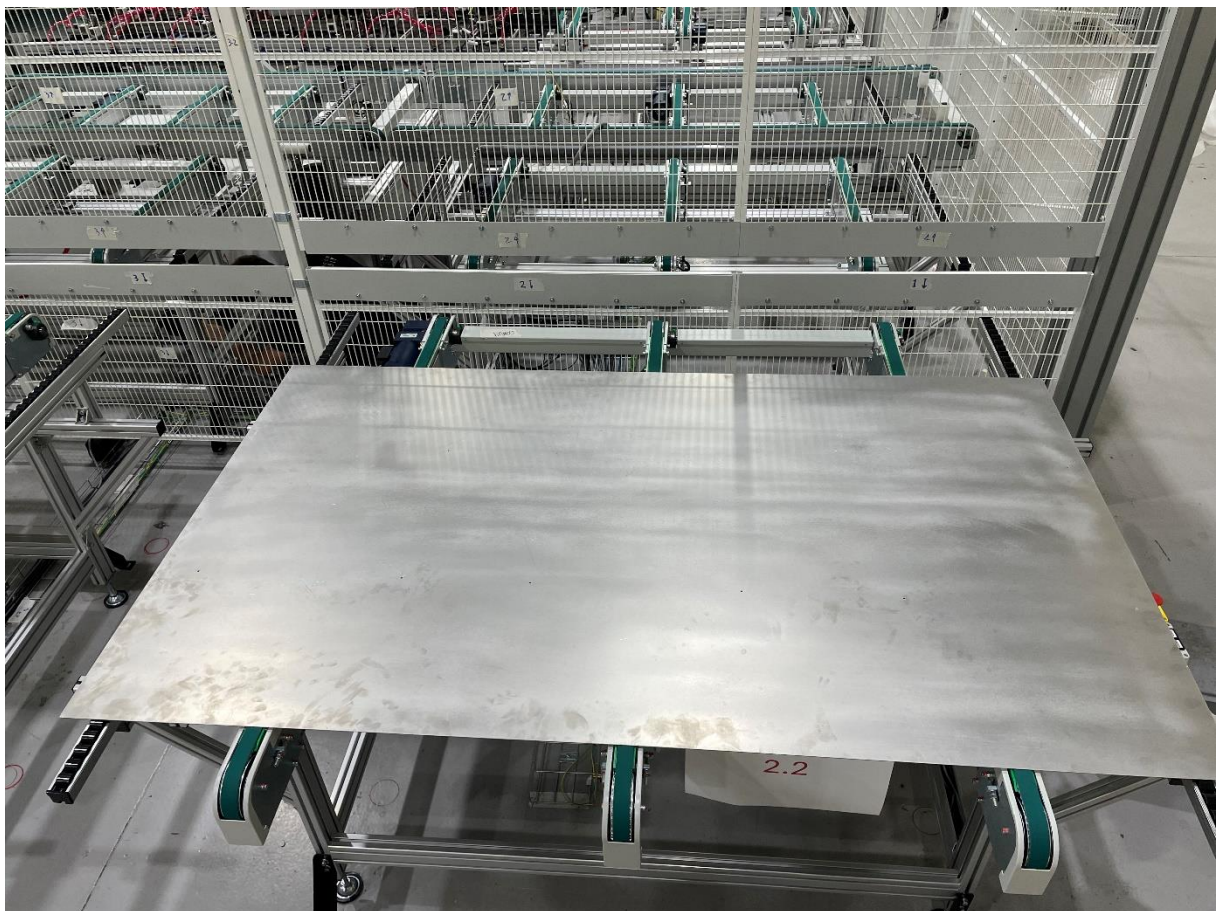
Figure 16 Example of a carrier over a conveyor
