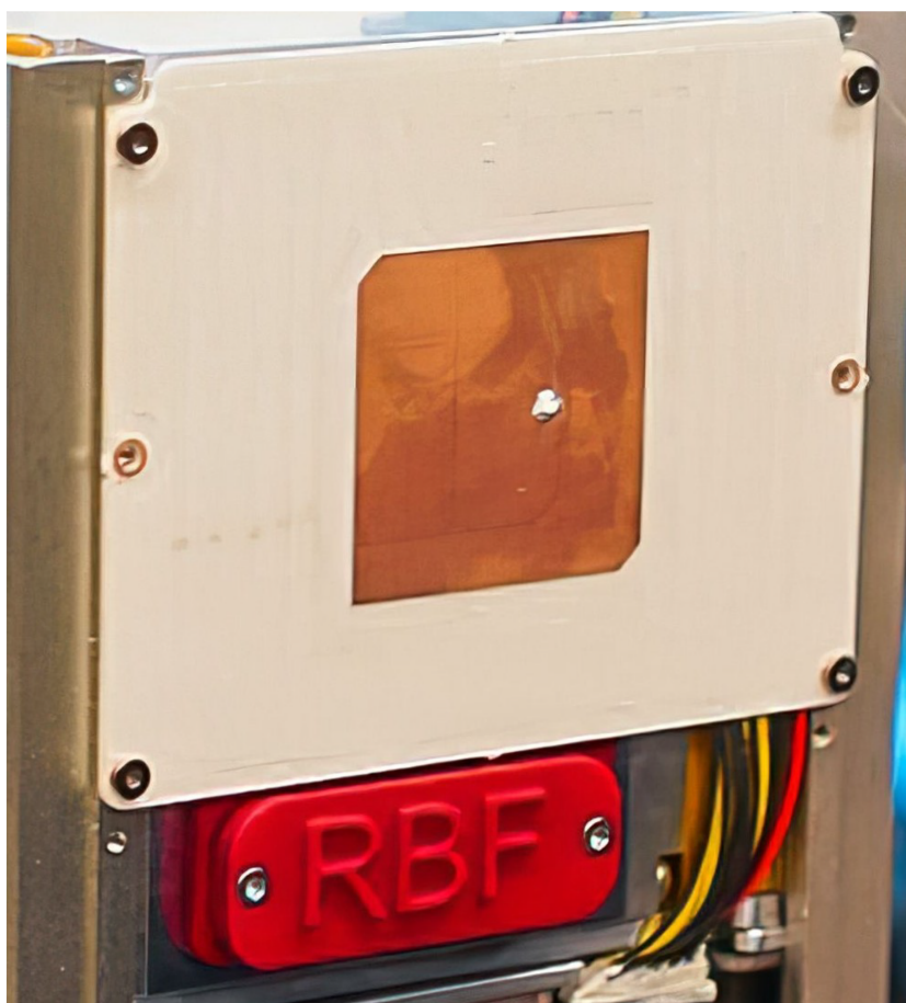
Figure 3.4: The patch antenna used for HSCOM of ESTCube-2. [24]
