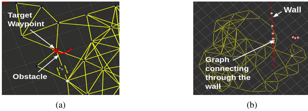
Figure 5.7: Problems with physical A* using odometry coordinates: odometry drift causing the target waypoint to be inaccessible around the obstacle (a), and the graph connecting through the wall (b).
