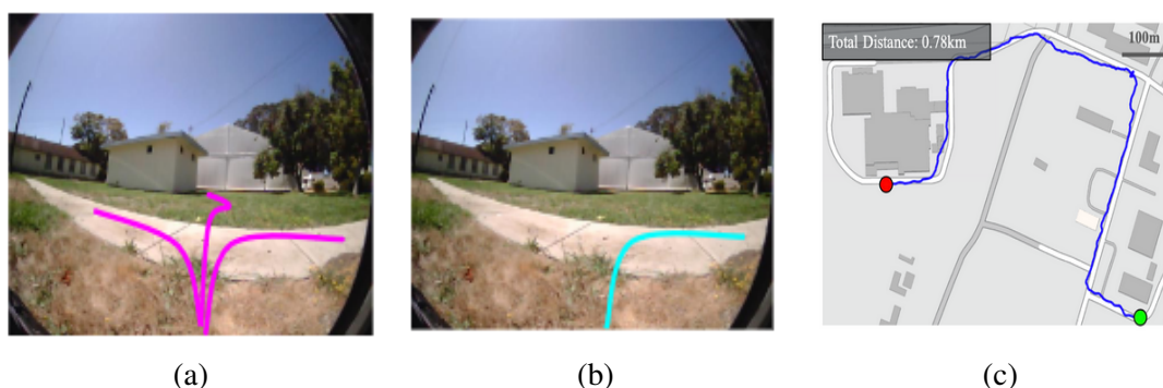
Figure 3.4: ViKiNG A* for physical search: Local planner sampled waypoints in (a), global planner selected waypoint from the waypoints proposed by local planner in (b) and the robot trajectory in one of the test locations of ViKiNG where global planner is conditioned over a road map in (c) [3].
