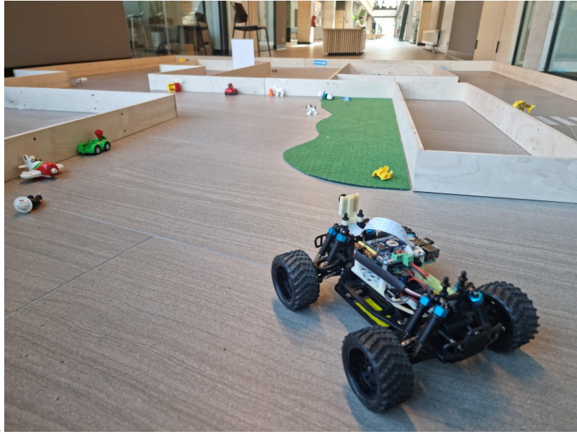
Figure 6: Indoor experimentation of self-driving capabilities of Donkey Car
