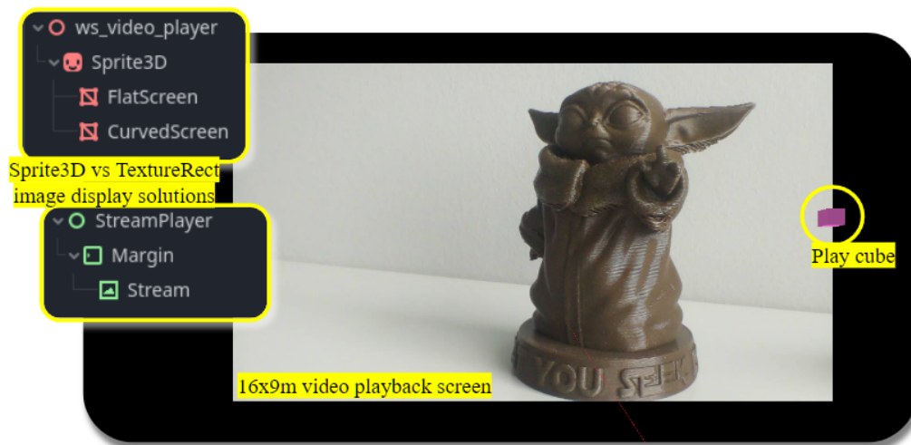
Figure 3.11: AR scene with a view from the player. The background stays black as pass-through is not available on PC. Highlighted cubes were added to the scene to exemplify how the scene can be made more immersive and interactive. Featured in the centre is a 16 by 9 m video playback screen.
