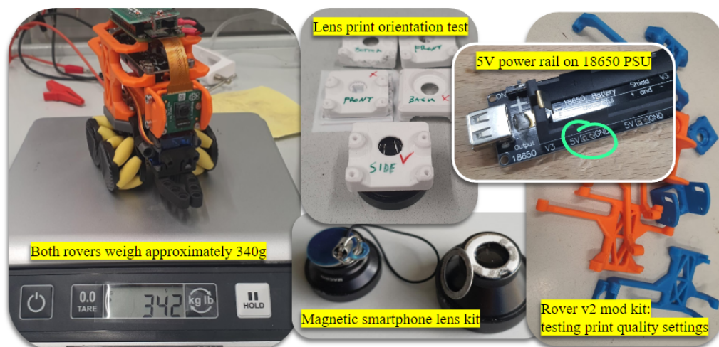
Figure 3.3: Printed part tests & breakout board planning. Rover v1 weighed ~342g. Rover v2's design process focused on the lens mount (top middle), lens placement and camera specifications, ensuring good image quality. A breakout board with a switch was added to control the 18650 PSU (top right) power rail.
