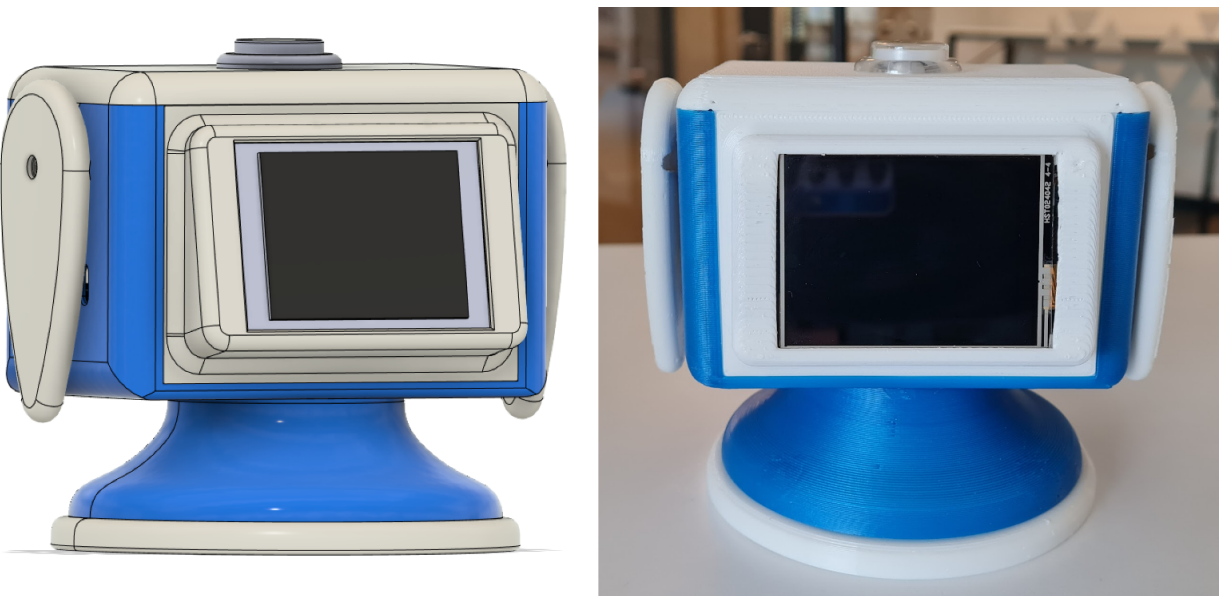
Figure 4.1: Side-by-side view of the CAD and the printed prototype of the RSC.
