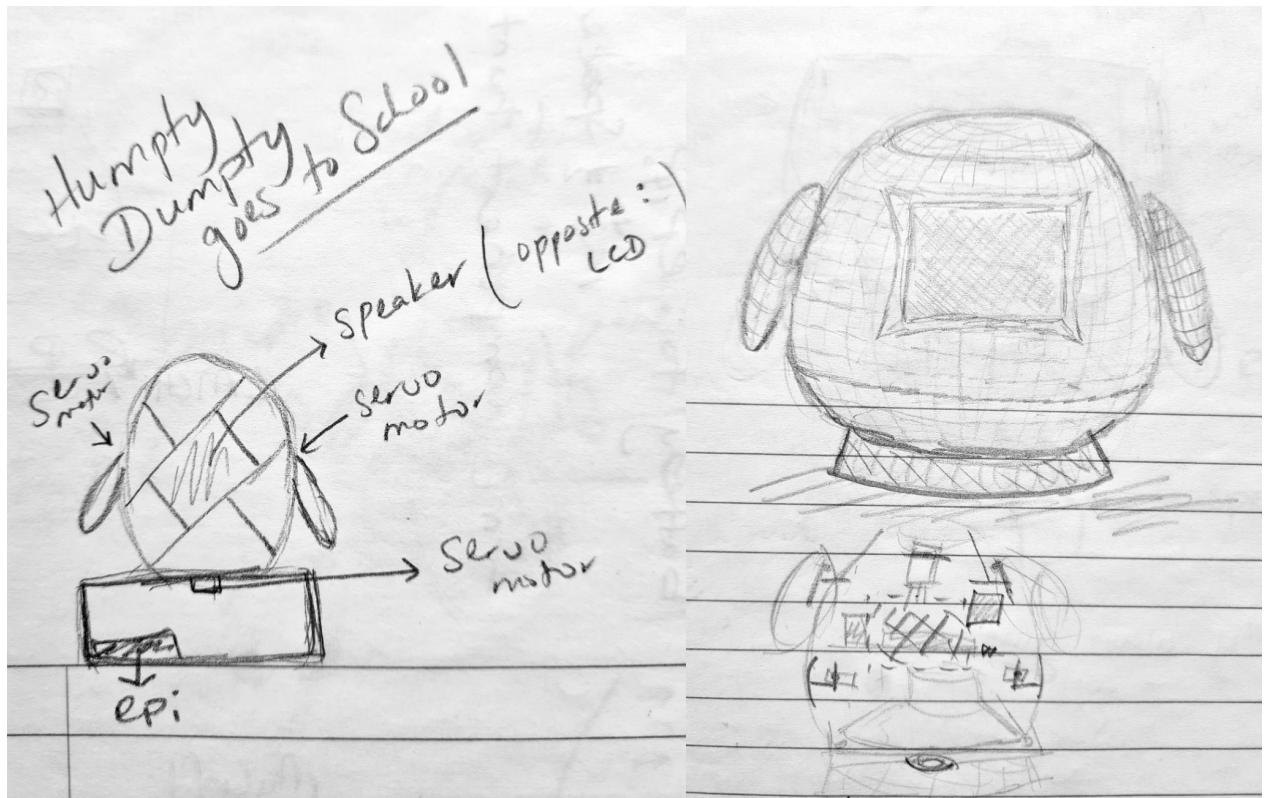
Figure 4.4: Initial design concept for a spherical robot body inspired by existing solutions. Due to challenges in housing all the components, the attempt to model this design was unsuccessful and earned the nickname 'Humpty Dumpty' due to its resemblance to an egg sitting on a wall.
