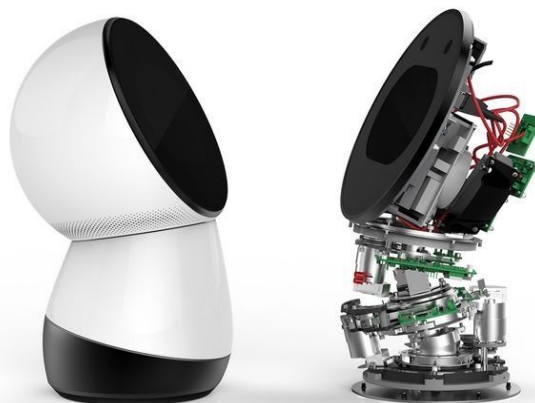
Figure 2.2: Jibo's external and internals [27]
