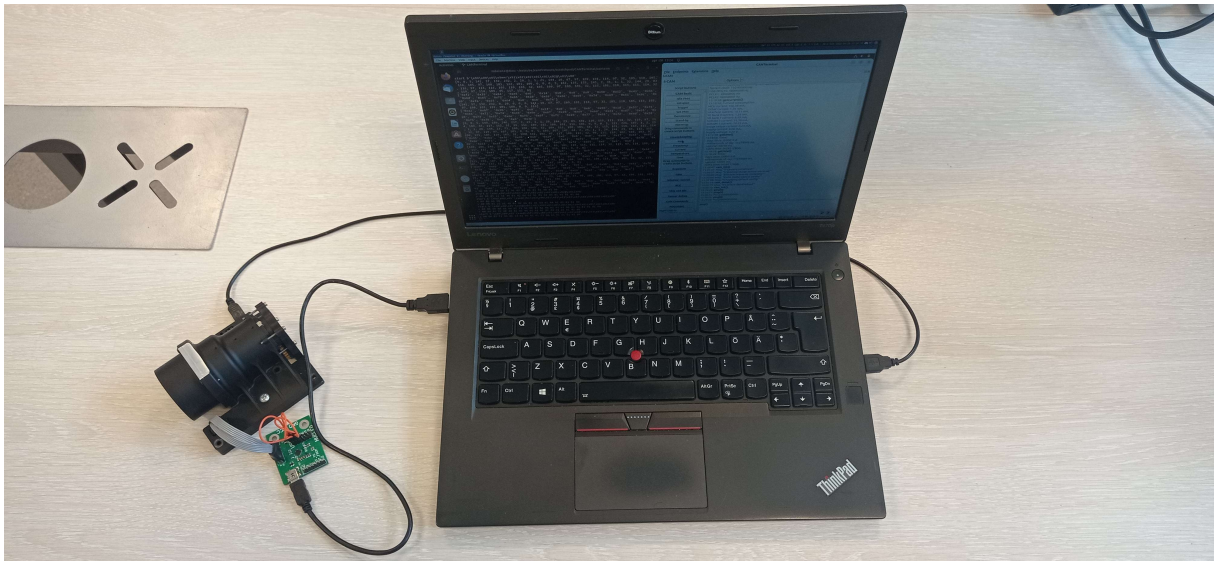
Figure 15: Testing the camera with the helper board. Both camera and the RS485 helper board are connected to the laptop.
