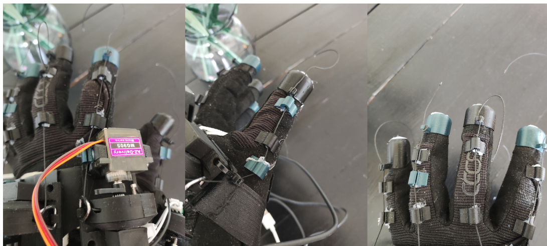
Figure 2.10: Second Glove Iteration Guide Nodes
