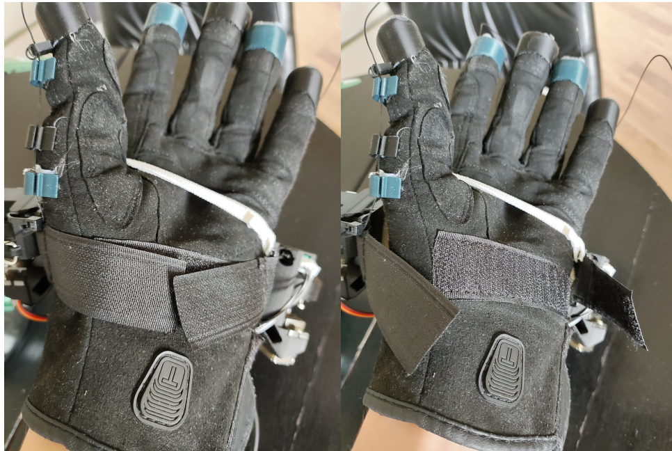
Figure 2.11: Second Glove Iteration Strap
