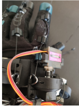
Figure 3.3: Rotated Cover to Put Tension on Metal Loop
