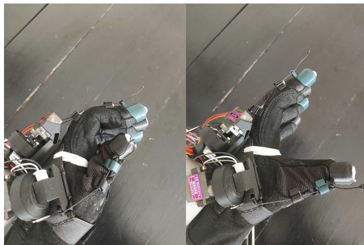
Figure 3.1: Problem When Fingers Were Not in End Caps
