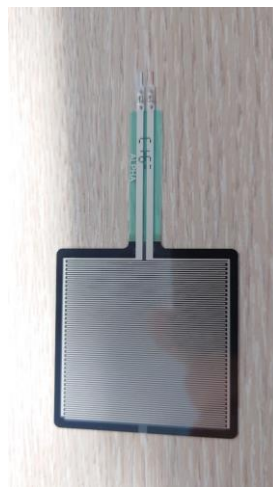
Figure 7. Thin film pressure sensor used on the corset
