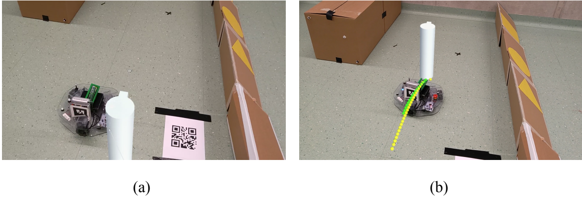
Figure 20: Unity application to control MR (a) before sending the command with goal object and QR code visible and (b) during movement with global trajectory (yellow) and local trajectory (green) visualized
