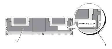
1 fully buffered DIMM
