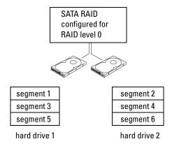
Another advantage of a RAID level 0 configuration is that it utilizes the full capacities of the drives. If you have two 120-GB drives installed, you have 240 GB on which to store data.
