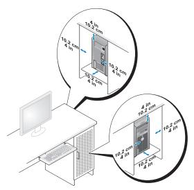
• If your computer is installed in a corner on a desk or under a desk, leave at least 5.1 cm (2 in) clearance from the back of the computer to the wall to permit the airflow required for proper ventilation.
