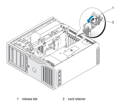
Press the card retention device back into its original position; push it down until it clicks into place.
