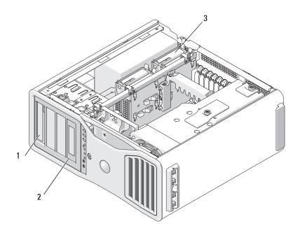
four 5.25-inch drive bays (can hold an optical drive, floppy drive, Media Card Reader, or SATA hard drive in a special drive case)
