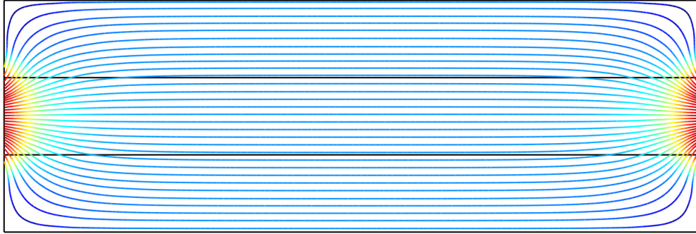
Figure 4: Streamlines in 2D. Flow enters from the right side and leaves from the left side.
