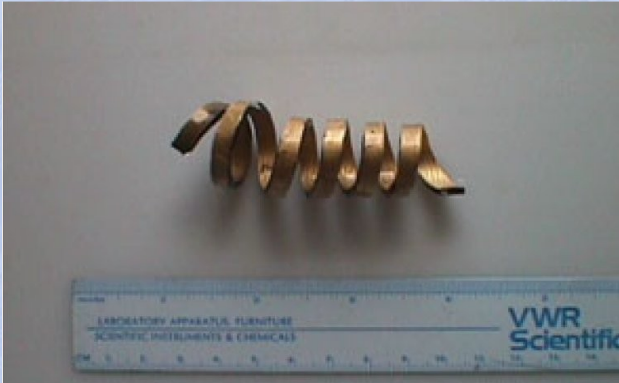
IPMC manufactured in a 3D shape Kim & Shahinpoor (2003)
