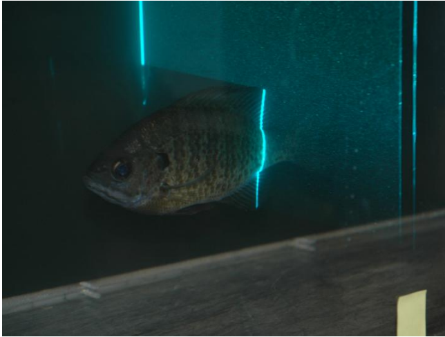
Figure 12. Photograph of a bluegill sunfish swimming in a flow tank intersecting a light sheet used to quantify pectoral fin flow in the transverse plane.
