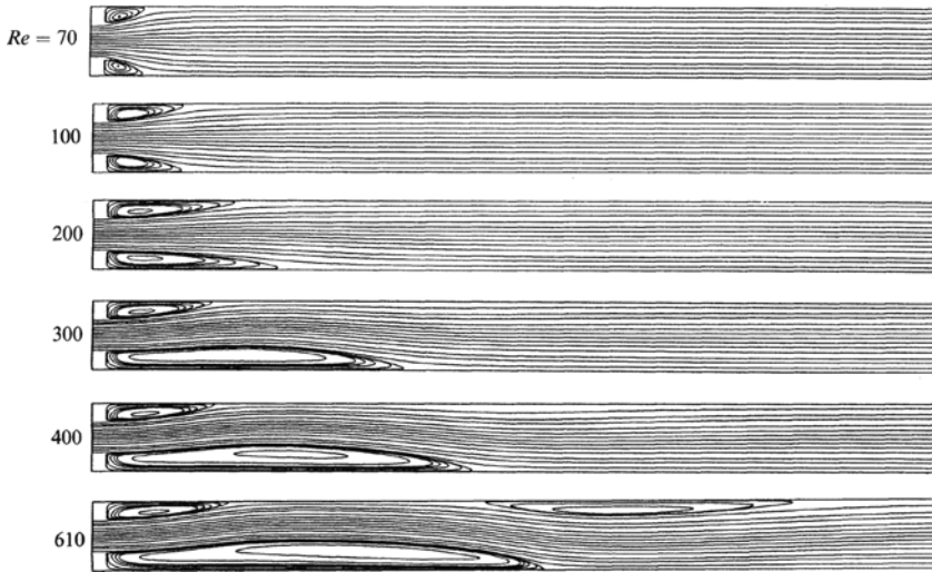
Fig. 7.6 Streamlines for the flow field of sudden channel expansion as a function of the Reynolds number
