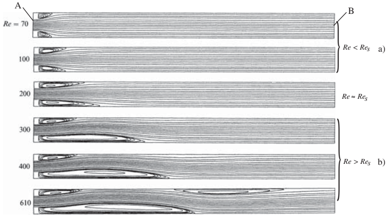
Fig. 17.11 (a) Two-dimensional plane channel flows with sudden expansion of cross-sectional area; (b) computation results with an asymmetry of the flow
